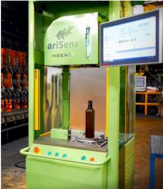
ariVolume aims to provide measuring bottle capacity at the HOT and COLD end.
